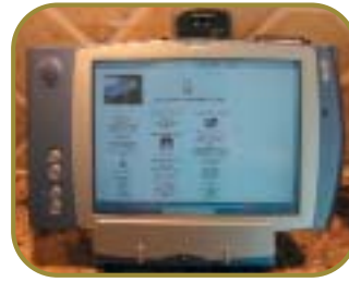
Hand-held wireless tablet, the AquaPAD is the web-appliance shared by family members to access household messaging, entertainment, and control functions.
